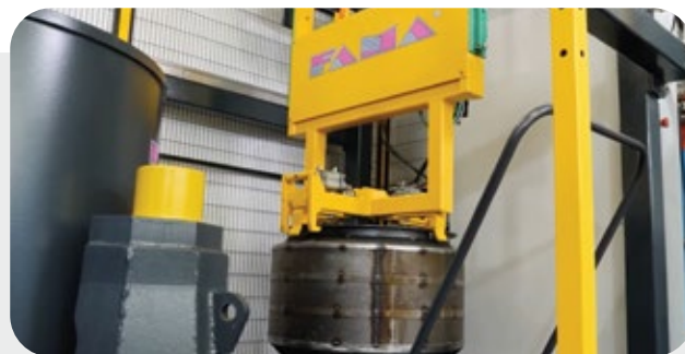
Automatic metal chip deoiling system with manipulator and removable basket centrifuge
